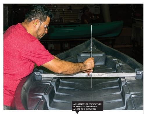
» manufacturing and made it more accurate and sophisticated. "All of our machines are computer-controlled," Swoger emphasizes. "Many of them are equipped with a feature called infrared thermometry, which allows us to control how long a part is kept in the oven or in the cooling station based on the temperature of the part rather than just the time. This is a great feature because it allows us to make much more consistent products."
